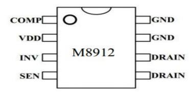
Figure 2. Pin configuration
