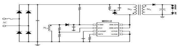
Figure 1. Typical application circuit for M8912
