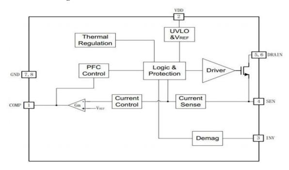
Figure 3. M8912 Internal Block Diagram
