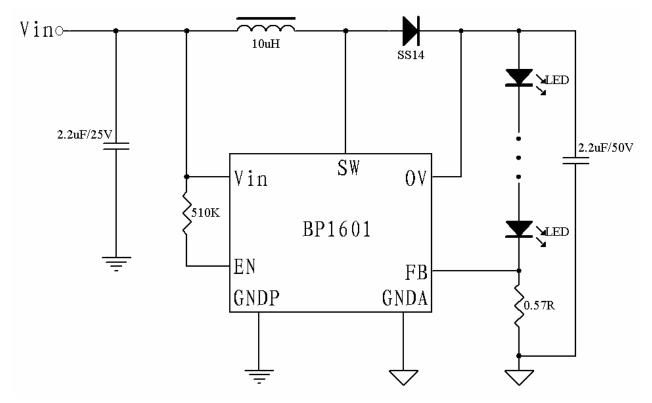
Figure 4 typical application circuit(7\*1W)
